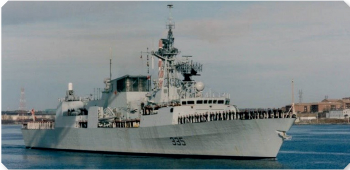
Canadian patrol frigate fitted with DRES Ball, 1986. The infrared signature was six to seven times better than the best available at that time.
