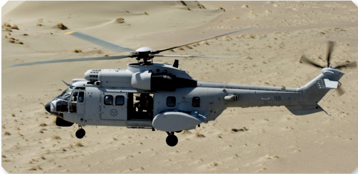
A Swedish Super Puma helicopter with infrared signature suppressor.
