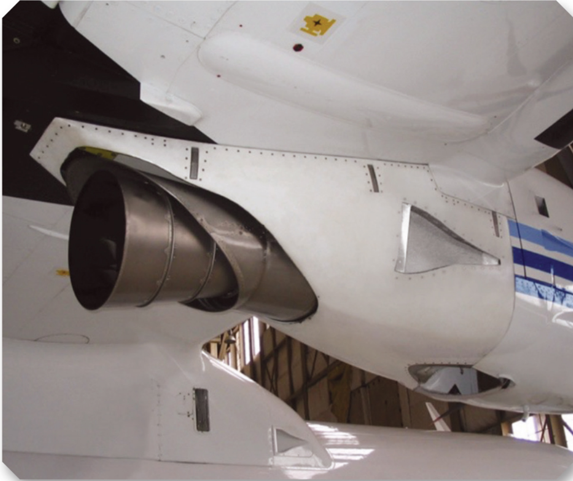
CN-235 transport aircraft fitted with infrared signature suppressor.
