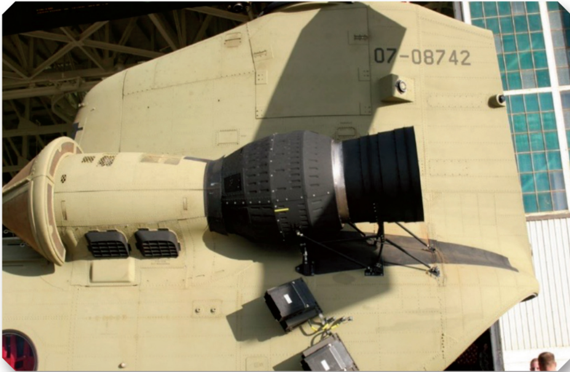
CH-47 fitted with infrared signature suppressor.
