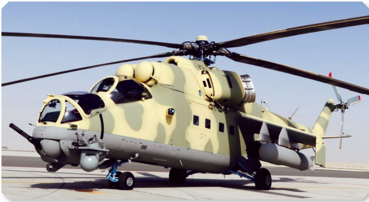
An Mi-24 helicopter with infrared signature suppressor.
