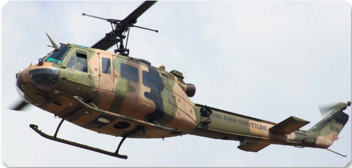
A Turkish Huey UH-1H with centre-body cooled tailpipe. This was our first big international contract.
